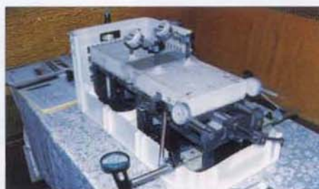
FIGURE 4 - TEST RIG TO SIMULATE CRACKING
