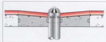
FIGURE 22 - BLOCK-OUT DRAIN USING VOICLAY BX WATERSTOP AT JOINTS
