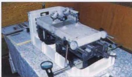
FIGURE 4 - TEST RIG TO SIMULATE CRACKING
